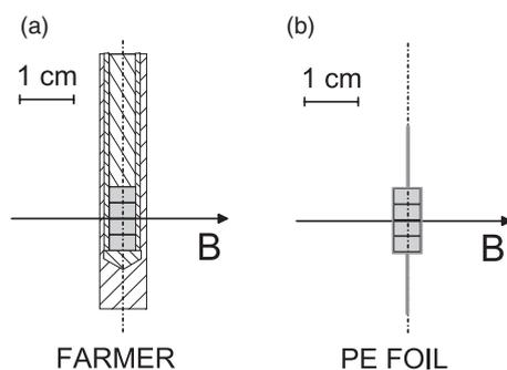
**Figure 1.** Different probes used—panel (a) detector with a PMMA holder fitting in a watertight sleeve for a Farmer chamber; panel (b) a detector shrink-wrapped in 0.2 mm strong PE foil. The capital B denotes the beam axis, the dash-dotted line indicates the symmetry axis of the detector.
