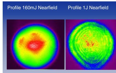
Pulse energy: up to 1J (lamp pumped)
