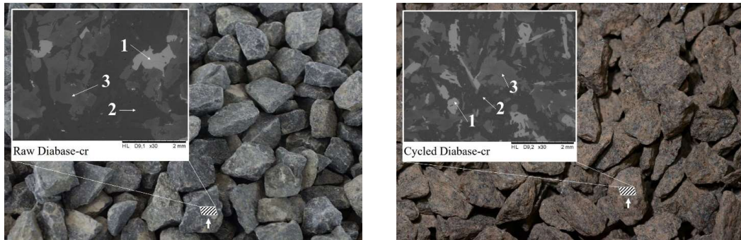
Fig. 8 Single-lens reflex camera and SEM imaging of raw and cycled diabase. Numbered areas in SEM images correspond to main minerals identified with their chemical composition in EDS [4].
